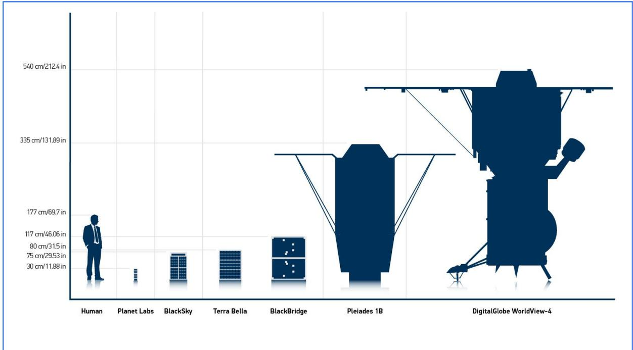
**Figure 1. Comparison of low-cost Planet Labs cubesats (left) with other remote sensing spacecraft (Digital Globe).**
