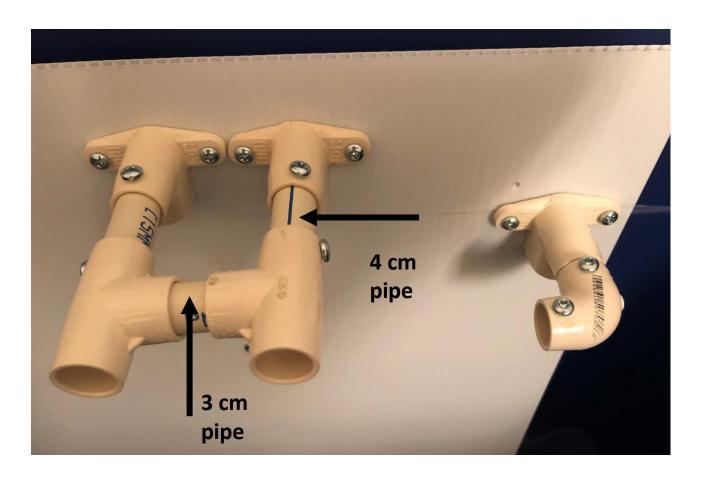
Attach the 4 cm pipe to the elbow and connect it to the Tee as shown in the picture. I recommend put some screws to secure the pipes to the elbows and tees. Connect both tees with the 3 cm pipe. I don't recommend put a screw on the 3 cm pipe because the sling tee needs to be loose, so the mechanism can work. Feel free to make this part better and let us know sharing your improvements. Don't forget to do the same in the other side.
