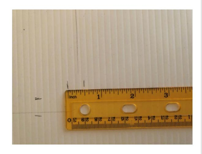
Drill a hole in each mark. You can use a screwdriver or something pointy to do the hole.
