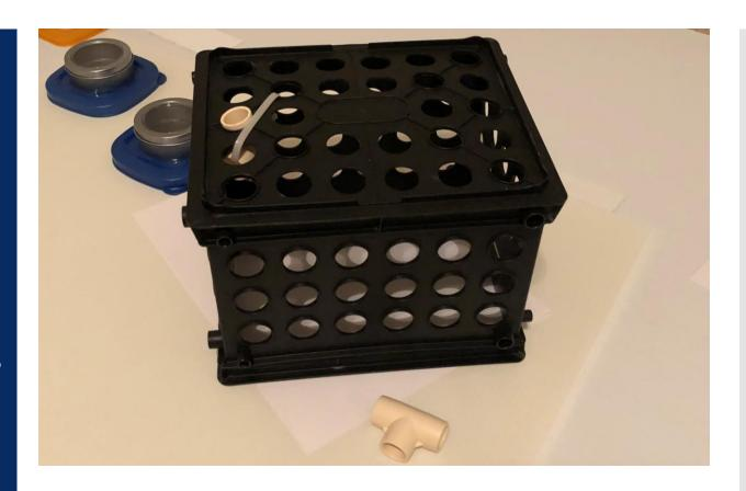
Take a CPVC Tee and insert the Tee with the middle hole pointing up in one of the holes of the crate next to the side. Take a cable tie and pass it through one end of the Tee to the other, so you can secure the Tee to the crate.
