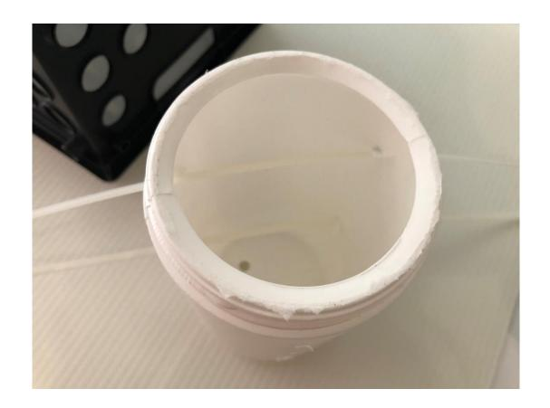
Open the lid of the container and pass 2 cable ties through the holes. You will be attaching that to the crate.
