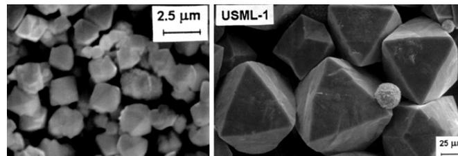
*Zeolite Crystals on the left were grown on earth. The ones on the right were grown in microgravity.*
