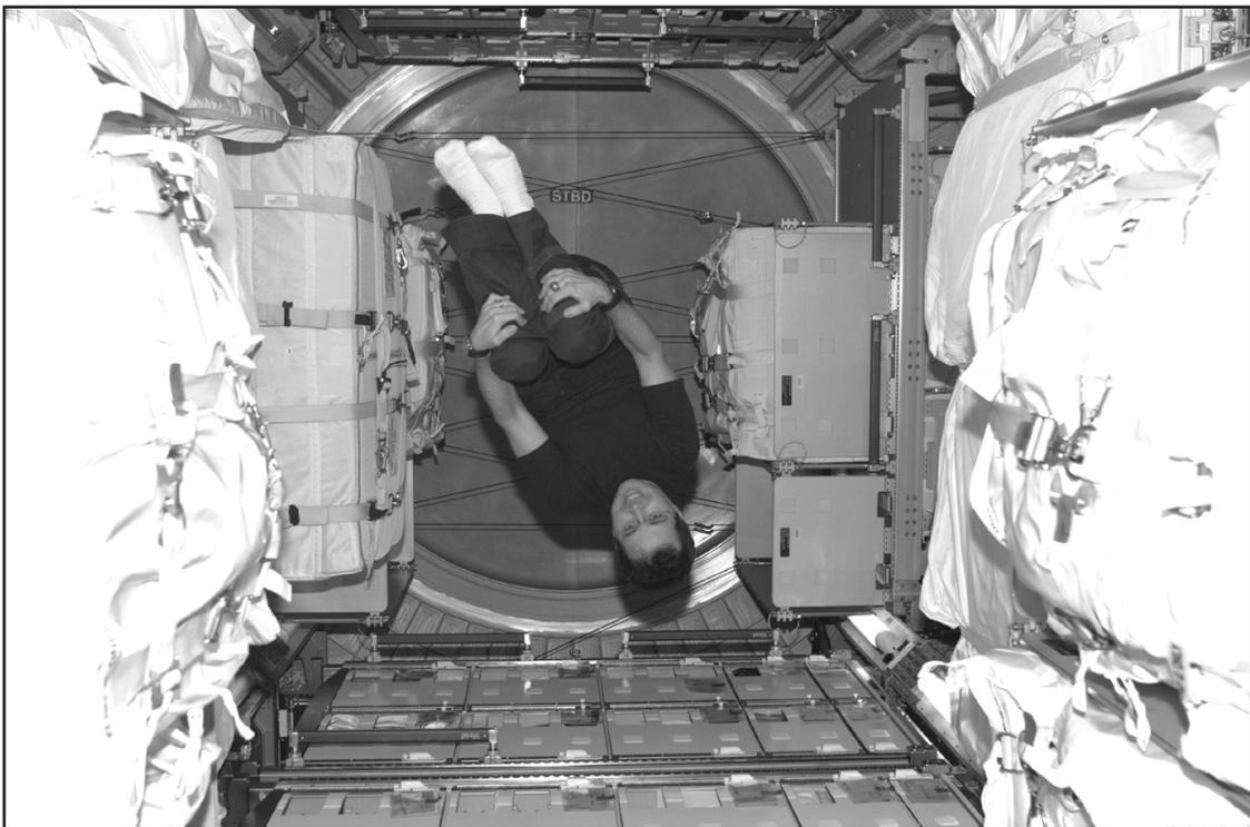
***A view from inside the Multi Purpose Logistics Module, Leonardo, which is a pressurized reusable cargo carrier to ferry supplies to the International Space Station. The MPLM was built in Italy.***
