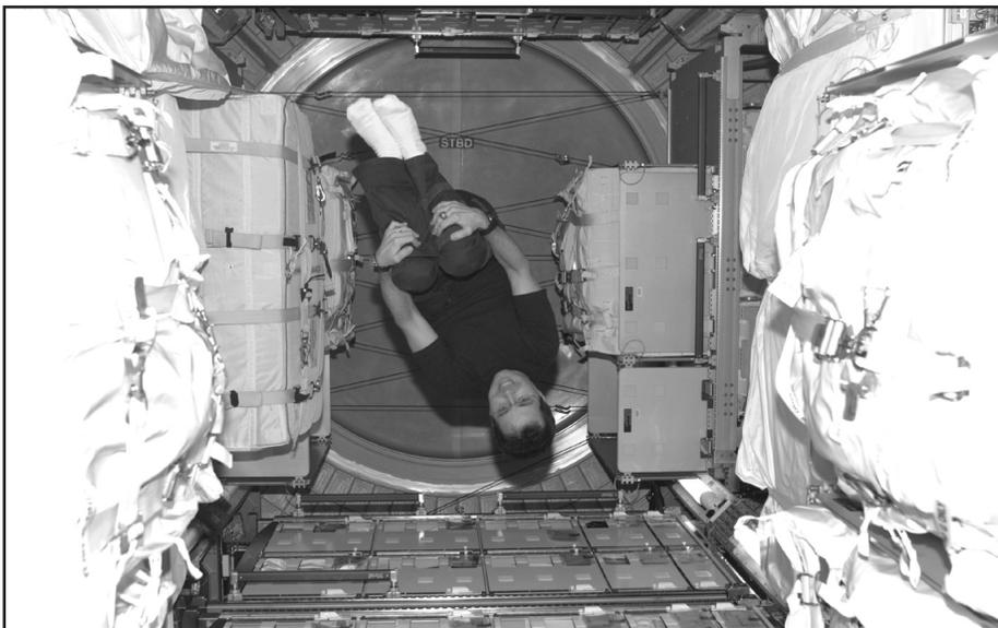
*A view from inside the Multi Purpose Logistics Module, Leonardo, which is a pressurized reusable cargo carrier to ferry supplies to the International Space Station. The MPLM was built in Italy.*
