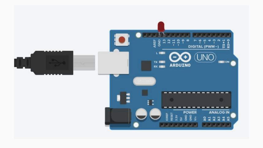
Add an Arduino Uno to the workspace and place an Led into the ports as shown (GND/13).
