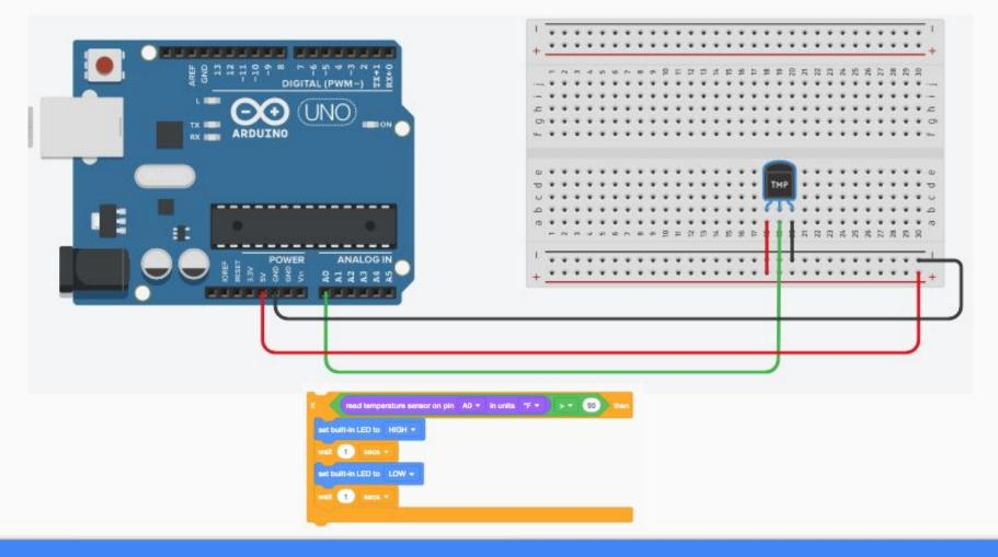
We can also add a temperature sensor and make an LED blink...like an alarm for high temperatures in a spacecraft.
