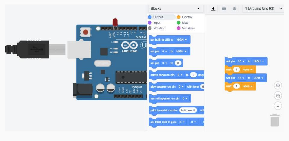
The built-in LED will be coded automatically. You can change the code to read "pin 13".
